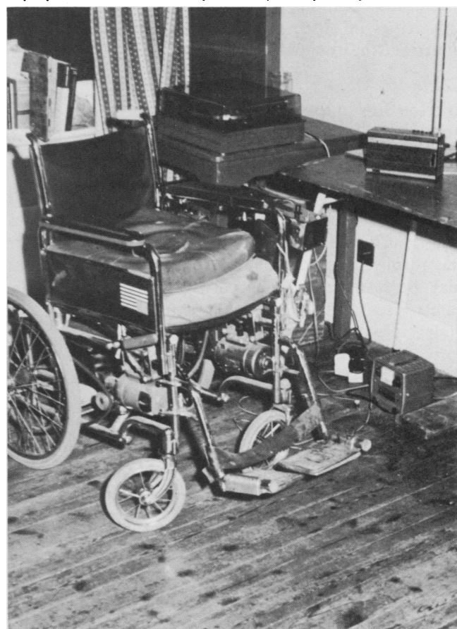
Figure 2. Carpet removed from study-bedroom, extra wall socket provided to enable electric wheelchair to be charged. (Student's hi-fi equipment has been specially adapted.)
