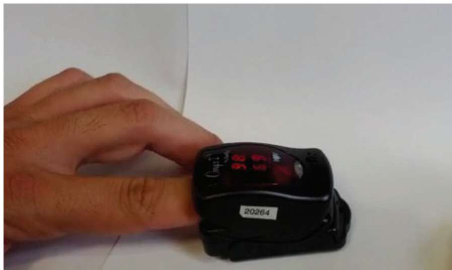
Figure 2. Pulse oximetry: pulse rate and oxygen saturation values are automatically sent via Bluetooth to the tablet computer.
